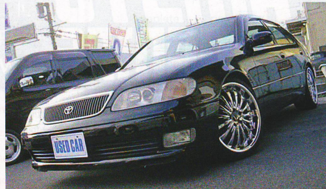
19-inch wheels fit okay, but you will have to remove part of the plastic inner guard
