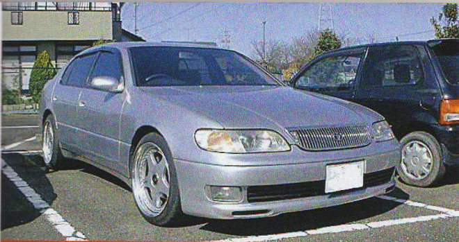
With the right offset you don't need the car too low for the wheels to 'fill-out' the guards
